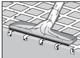
The hard floor nozzle is excellently suited for cleaning hard floors with crevices and joints. In order to clean crevices and joints most effectively, the nozzle must rest completely on the surface. To clean coarse soiling, it may be helpfully to angle the nozzle slightly.
