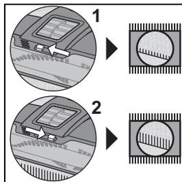
The turbo brush is ideal for cleaning animal hairs and straightening the carpet pile. *Caution: only clean non-delicate surfaces with the turbo nozzle. Otherwise there is a risk of damage.* The speed of the rotating brush roller can be adjusted with the slider:
