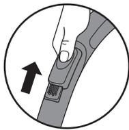
If curtains or other objects are accidentally suctioned, quickly open the slide vent to release the objects again.
